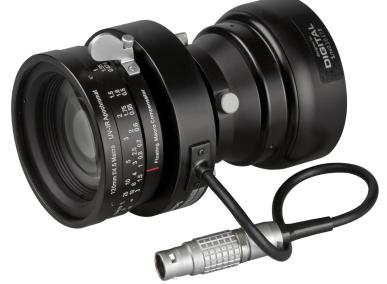
Hyperspectral Macro Apochromat shown above with manual Copal-0 Shutter and at left with digital shutter. Digital shutter may be powered and controlled over USB using Photoshoot Control software or other applications. While the digital shutter integrates seamlessly with MegaVision's digital backs and is incorporated into the EV camera, MegaVision PhotoShoot Control software enables shutter operation with other digital backs and in other capture environments.
